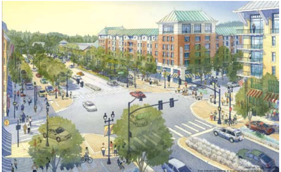
Instead of being a conventional strip-like arterial barrier between downtown’s historic core on the east and new mixed-use infill developments on the west, the five-block “multiway boulevard” segment of SR-527 will subdivide its width into arterial lanes in the center, wide sidewalks with parking and slow lanes on the sides, and multiple rows of trees.
