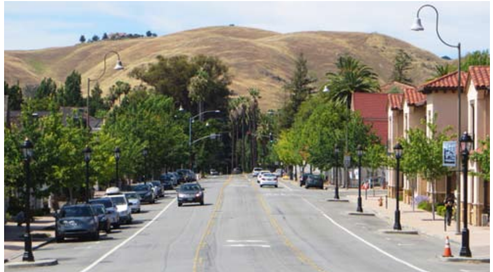
Mission Boulevard’s pedestrian scale was strengthened through placement of new decorative post-top streetlights between parked cars to visually “pinch down” the apparent street width for drivers and widen the pedestrians’ perceived areas.
