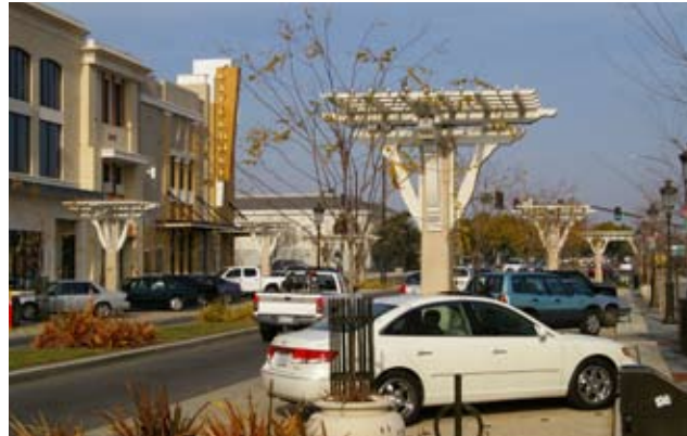
The wide, auto scale 4 lane arterial street was reduced to two lanes. The proportions of the street width were made even more pedestrian-friendly with the introduction of freestanding trellis structures and street trees within parking lanes. The wisteria-clad trellises were combined with extensive landscaping and existing bluestone paving to introduce a "winery patio" character into downtown.
