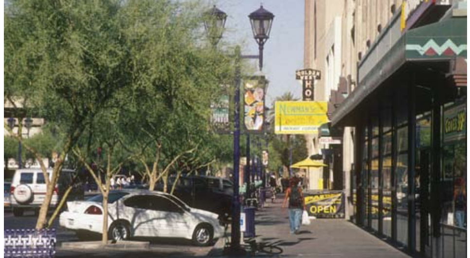
Monroe Street's pedestrian environment has been transformed with the introduction of coordinated furnishings, trees placed in the parking lane, angled parking, and two-way traffic. The design has drawn in new shops.
