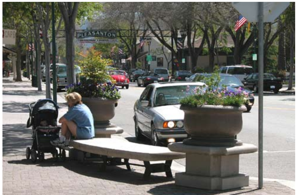
Custom furnishings were designed to complement Pleasanton's mix of historic architecture and to be substantial enough to provide pedestrians the impression of being buffered from traffic. Unit pavers were focused at corners and crossings, with less costly pigmented stamped concrete at sidewalk segments in between.
