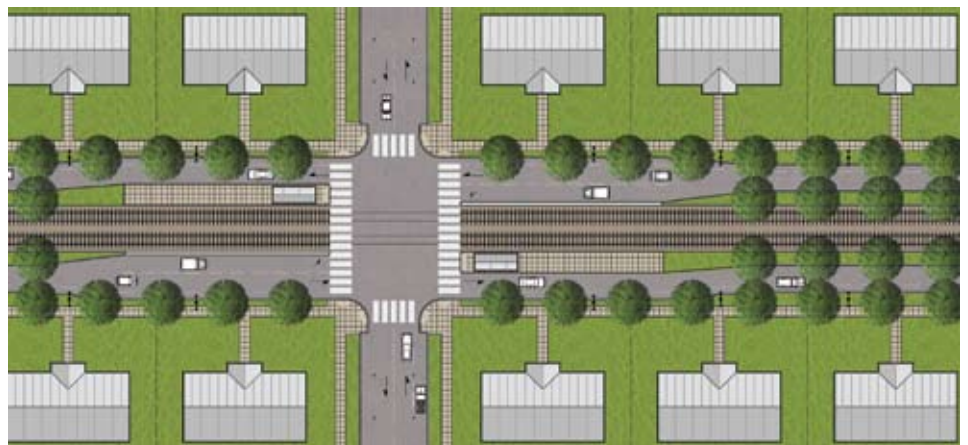
Conceptual streetscape showing a linear parkway is converted to a light rail or bus rapid transit lane.
