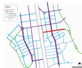
Street Hierarchy. In lieu of the usual single large arterial, vehicular circulation is served by a network of through-streets that form the framework for development of the new district. All streets in the hierarchy are designed to accommodate pedestrians, bicyclists, transit-riders and motorists.
