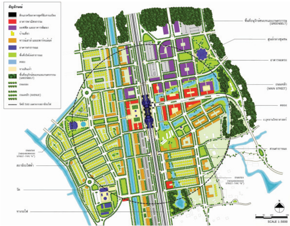
District Master Plan (above). The mixed use district orbits around the train station and a main street that extends eastward from the station toward Thammasat University. District quadrants are composed of residential and employment neighborhood sub-areas that center on civic spaces and civic buildings.
