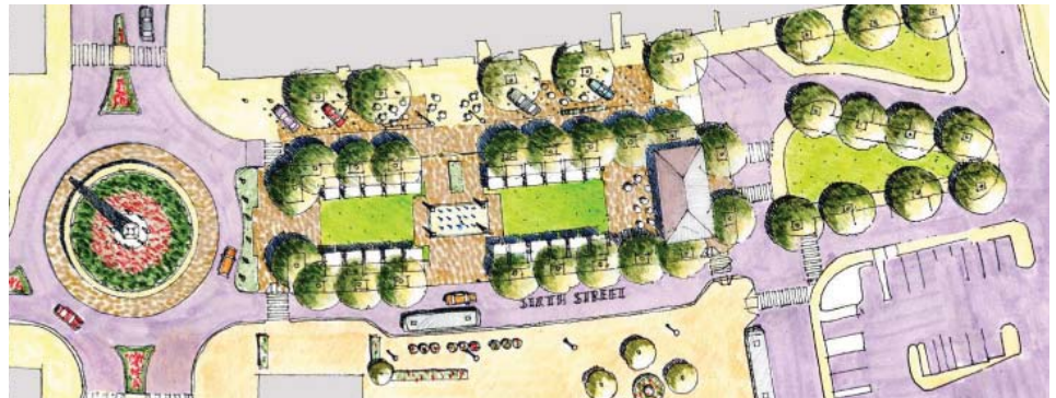
Illustrative plan view of roundabout at Central Ave. and 6th St. intersection, fountain plaza and lawns infilled onto former parking lot site, westbound 6th street lane restored along north side shops and angled parking with "flexible zone" dining areas, future plaza pavilion east of plaza, and eastbound 6th St. lane, Transit Center building and drop-offs at south side.
