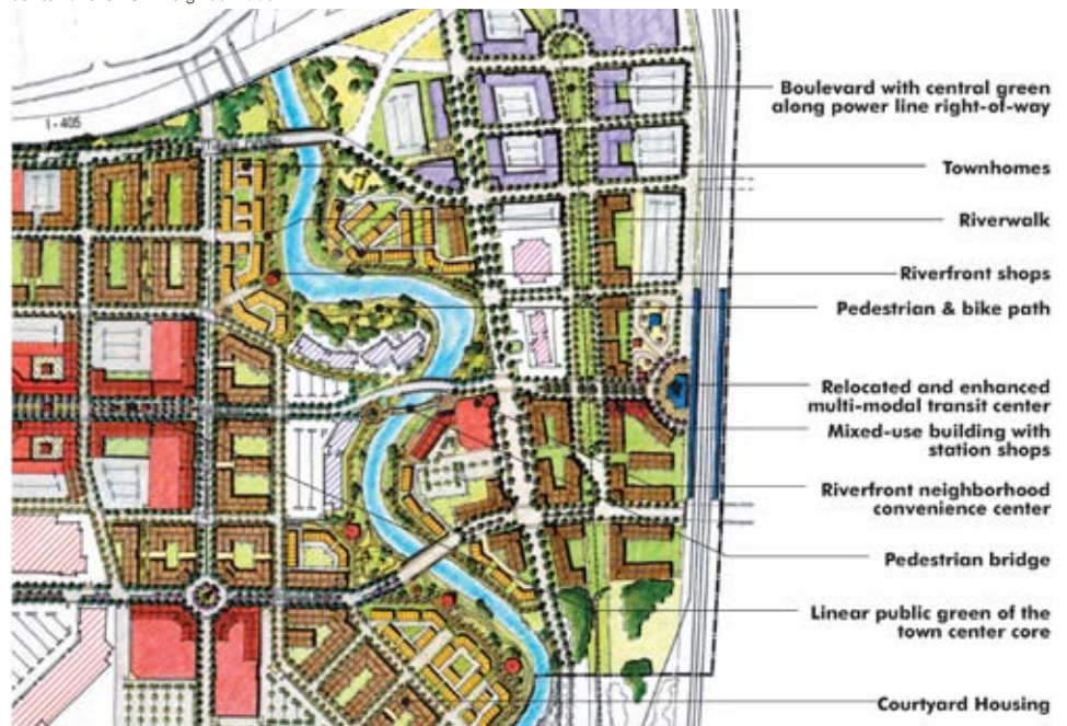
The relocated and redesigned transit center forms the terminus of a new sequence of pedestrian-scaled streets lined with a mixture of street-fronting high density buildings, leading to riverfront townhomes, and ultimately to a new main street and the core of the regional mall
