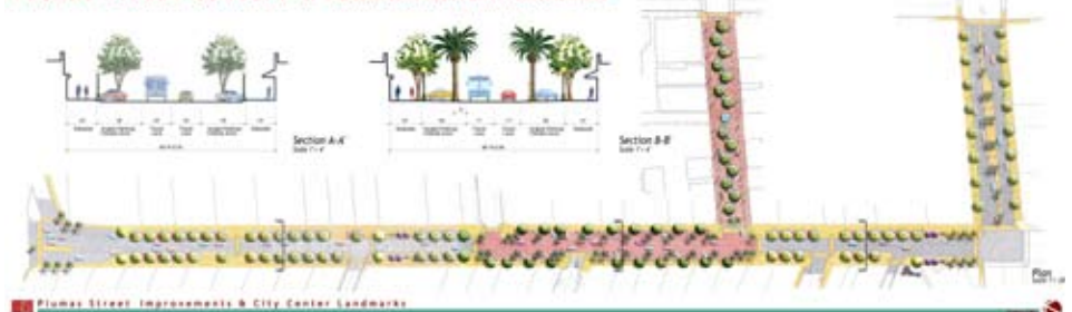
Illustrative Streetscape Concept Plan of Plumas Street's 7 block, nearly 2,000 foot length. The design concept contained street tree plantings within angled parking lanes throughout, special treatments of its northern and southern downtown entries, accenting of entries and plaza areas with date palm trees, and special streetscape concepts for side streets.
