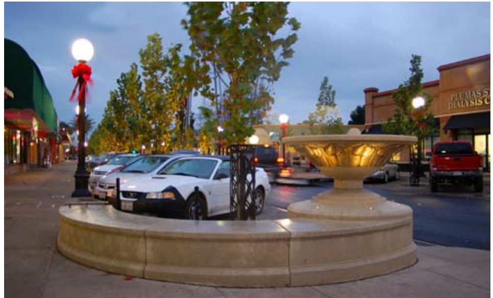
Custom-designed street furniture at every corner "bookends" diagonal parking, creates seating, and adds a signature decorative planter bowl for colorful flowers. The street is lit with high quality, energy efficient induction and LED lighting. Angled parking spaces are "flexible zones" that will be convertible to outdoor dining areas when city regulations permit.
