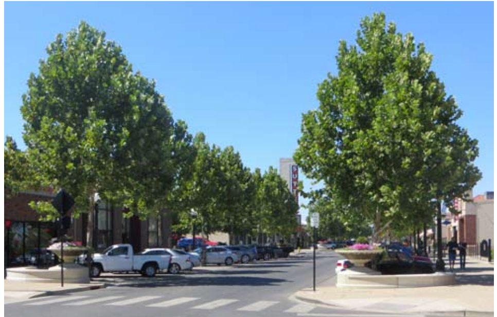
AFTER: Planting of canopy trees between parked cars, widening of sidewalks, shortening of crosswalks, and introduction of special furnishings and flower plantings has created abundant shade, helped to slow down previously 40 mph traffic, and dramatically changed the "look and feel" of the street from auto-dominated to pedestrian-friendly.
